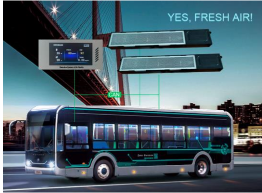
4. Nano filter & purifier system on bus' air conditioner
